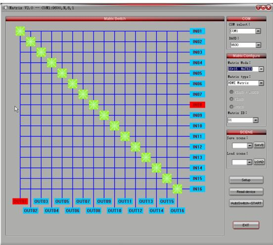
Software open the last saved serial port and baud rate. If any error dialog box appeared, please check the current device connection port and baud rate. Default baud is 9600, device ID is 1.
